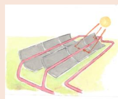
Solar collector used to heat a fluid
